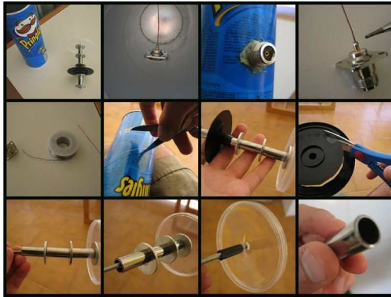
Figure 9.1: The famous Pringles 2.4 GHz antenna. Photo by otakon86, Source: www.flickr.com/photos/beakman/225399389/ , Creative Commons BY_NC_SA license.
