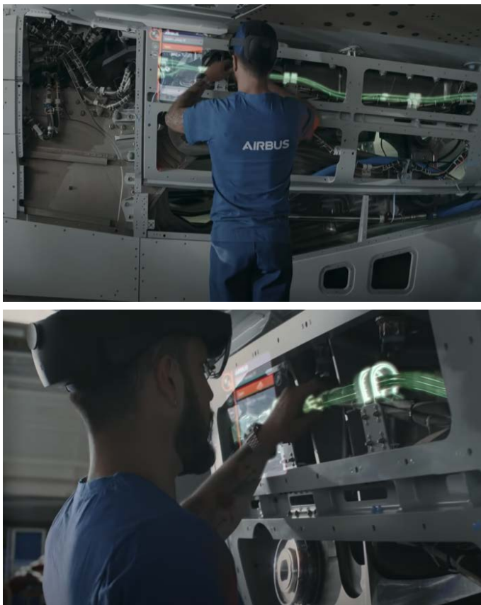
Fig. 10 a,b: A case study conducted by Airbus seeks to combine the construction site and instructions into a joint perceptual space by eliminating the offset between image and object (Microsoft Inc., 2019).
