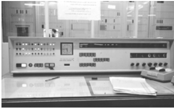
Fig. 1. The operator's interface. Computer SEL ER56 at Computing Centre, University of Stuttgart 1965. We see dials (lower right) and push buttons to get at specified data. Through the glass in the background some of the hardware
