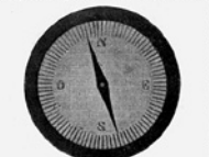
FIG. 2.—Photograph of a compass steel and needle completely enclosed in a metal case.
