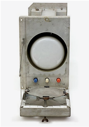
5 The Manchester Mark 1 Williams tube with the pickup plate.
