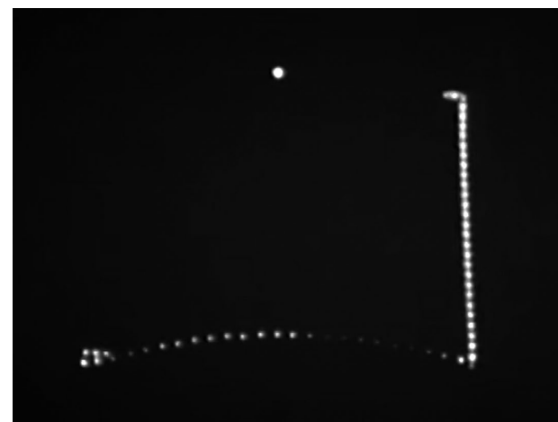
8 Trajectory of a rocket (without afterglow). The x-axis of the coordinate system is slightly curved on the right display. The dot of light (the rocket) is located at the highest point, the apex of the trajectory. The right bar indicates the velocity of the rocket.
