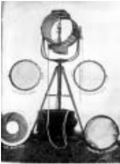
Fig. 2.12 – An American Sunlight arc lamp with its accessories.
