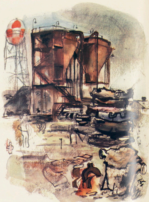
Slag from production of ferroalloys at Carbide's mammoth new Marietta, Ohio, alloy works is tapped out into troughs, broken down into smaller chunks by the use of high-pressure streams of water, and finally dried with heat in these "dewatering bins" before being reprocessed to extract any residue of metal.
