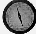
FIG. 6.—Photograph of a compass steel and needle completely enclosed in a metal case.
