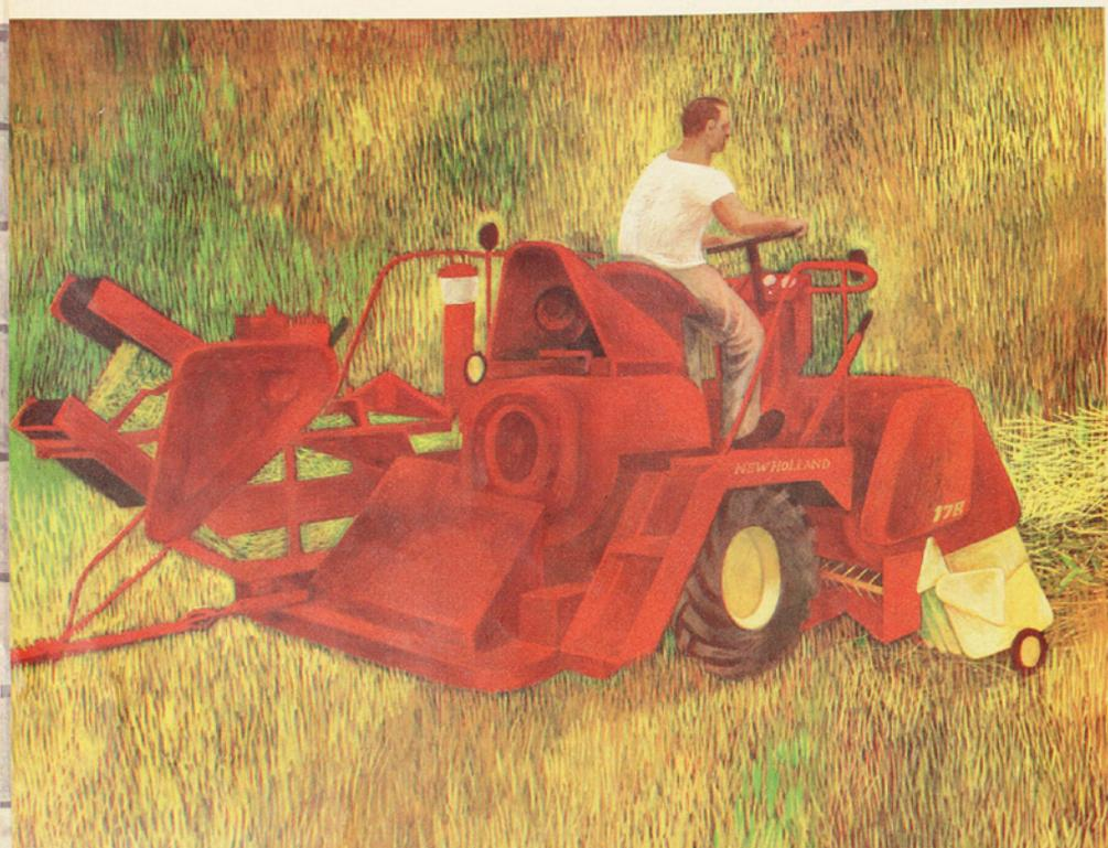
Self-propelled baler (with twine or wire tie) is at the head of the New Holland division's line of agricultural implements. The machine shown here is equipped with New Holland's new baler thrower, which automatically tosses big or little bales into pickup. This Sperry Rand division makes nearly all kinds of grainland farming machinery except tractors, plows, and other non-profit items. It consistently produces profits.
