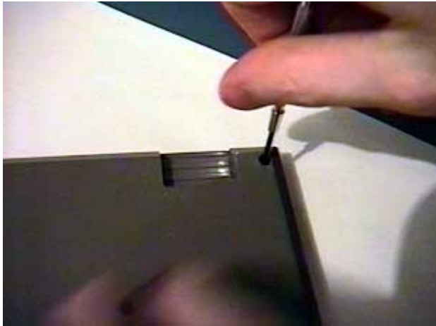
Here I am unscrewing a Mario Brothers Cartridge.
