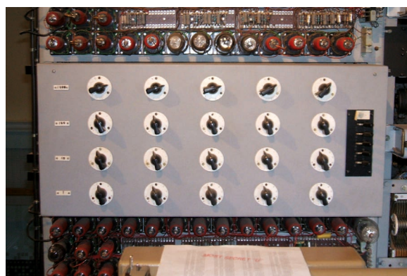
Fig. 25: Threshold controls set the criteria used to selectively suppress printing of totals (TNOC reconstruction). Photograph: Mark Priestley.
