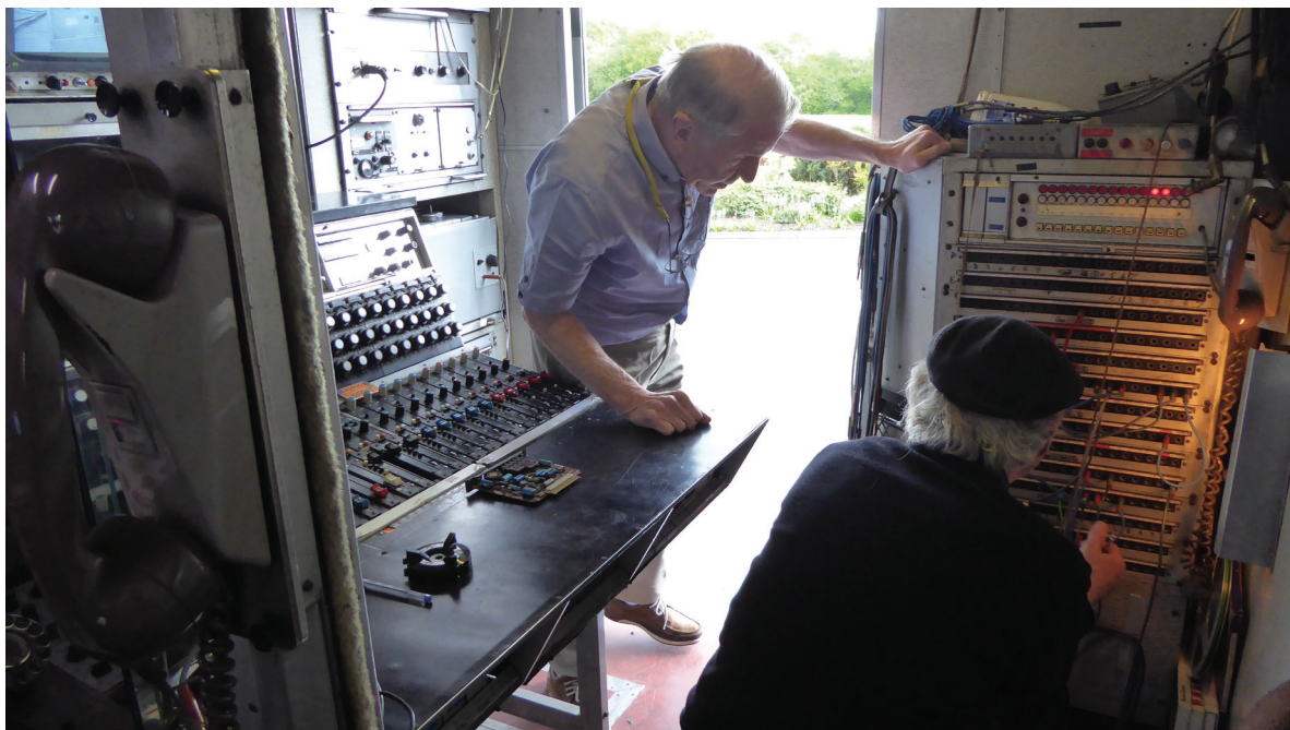
Figure 5. Ken Osbourn and Doug Whittaker work over the patch bay used to connect the numerous inputs and output within the OB scanner.
