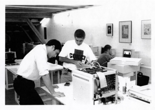
Figure 4. MIDE team is assembling a photocopier machine's Interface Processor Unit. ©MIDE documentary archive
