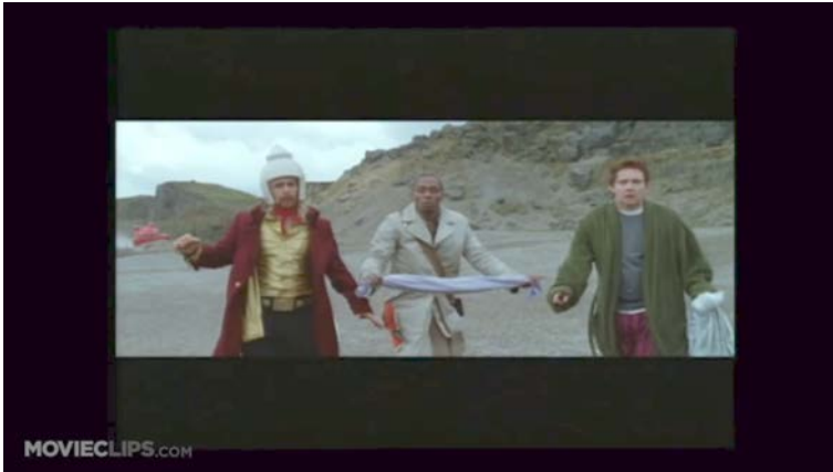
[Figure 3] Screenshot from a trailer for The Hitchhiker's Guide to the Galaxy (2005) circulated on YouTube, showing traces of multiple reformattings. The image originated with an anamorphic widescreen aspect ratio of 1:2.39. My brief examination suggests that this trailer may have been digitized into DV NTSC format, erroneously captured without correcting for DV's narrow pixel aspect ratio of 0.91 (thus stretching in width) and letterboxed into a 3:2 frame, subsequently letterboxed again into a 4:3 frame and finally pillarboxed for YouTube into a 16:9 frame.
